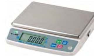
weighing scales – to measure weight in grams
